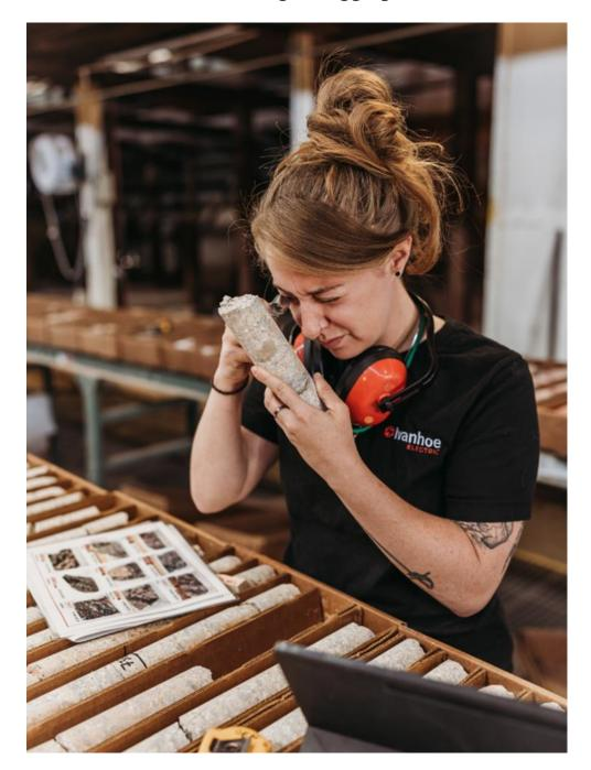
In early October, the Santa Cruz Project introduced on-site scanning of drill core utilizing cutting-edge technology developed by GeologicAl of Calgary, Alberta, Canada. The system utilizes several components including: Light Detection and Ranging ("LIDAR") scanning, X-Ray Fluorescence ("XRF") chemical analysis, hyperspectral analysis for mineral identification, high-resolution core photography and geotechnical data collection and analysis tools.
