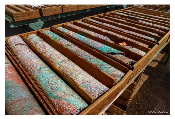
Prior to sampling drill core for assays, holes receive detailed geotechnical evaluation using rock quality designation, logging of whole core and mapping of structural features using downhole acoustic televiewer surveys. This data is essential for understanding the engineering characteristics of the rocks influencing potential mine design.
