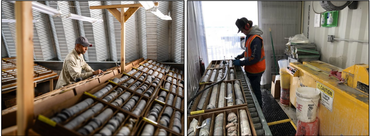
Figure 9-1: Drill core logging and cutting/sampling in progress at the core facility.
