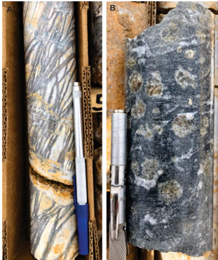
Figure 7-7: Drill Core Samples from Hole DDH2012-02 (completed by Applied Minerals) of (A) Intense Carbonate-Quartz Veining at 175 m Downhole Depth and (B) Pyroxene Skarn at 370 m Downhole Depth
