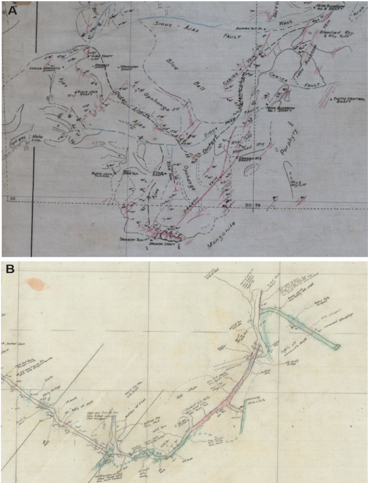
Figure 6-2: Examples of Historical Surface Mapping and Underground Geology Maps (A) a Surface Geology Map around the Dragon Mine (1 to 800 ft scale) and (B) Geology Map of Underground Workings at 300 level of the Iron Blossom Mine (1:400 ft scale)
