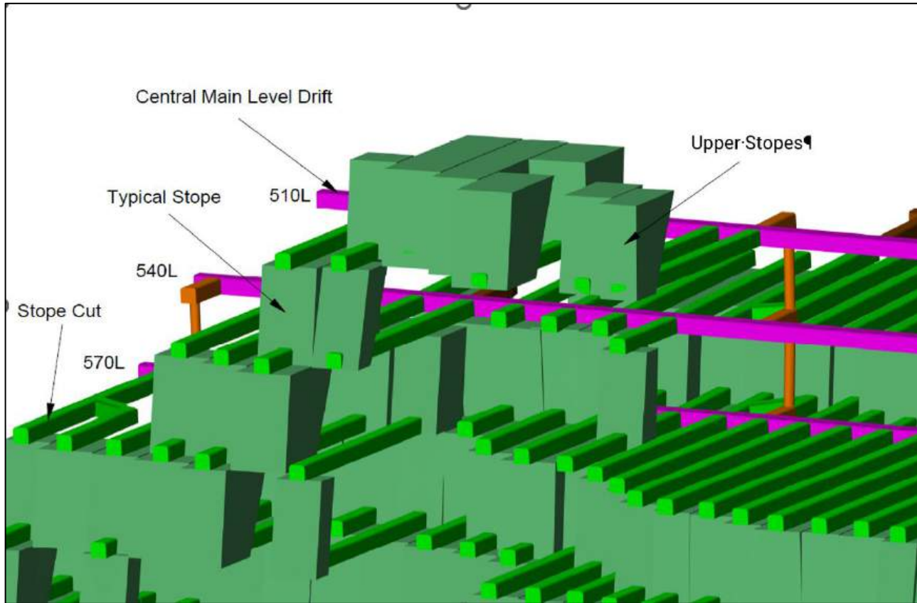
Figure 13-4: Transverse Longhole Stopping in the Santa Cruz Orebody (Looking Southwest)
