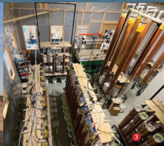
IMAGE 1: Hydrogeological drill testing. IMAGE 2: Vibroseis truck for 3-D mapping of mine geology. IMAGE 3: Column leach tests at Blue Coast Research Ltd. laboratories in British Columbia, Canada to support ongoing Preliminary Feasibility Study metallurgical studies.
