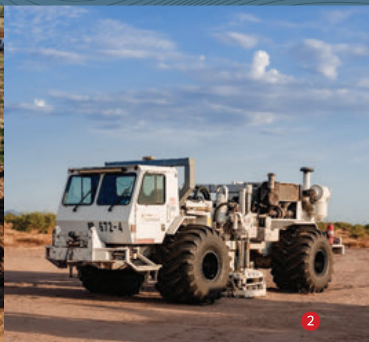
IMAGE 1: Hydrogeological drill testing. IMAGE 2: Vibroseis truck for 3-D mapping of mine geology. IMAGE 3: Column leach tests at Blue Coast Research Ltd. laboratories in British Columbia, Canada to support ongoing Preliminary Feasibility Study metallurgical studies.
