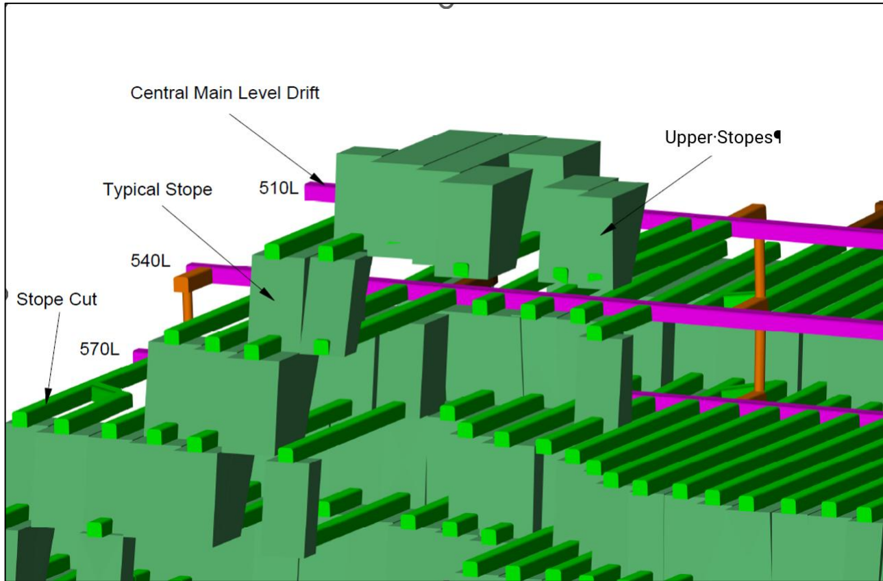
Figure 16-4: Transverse Longhole Stopping in the Santa Cruz Orebody (Looking Southwest)
