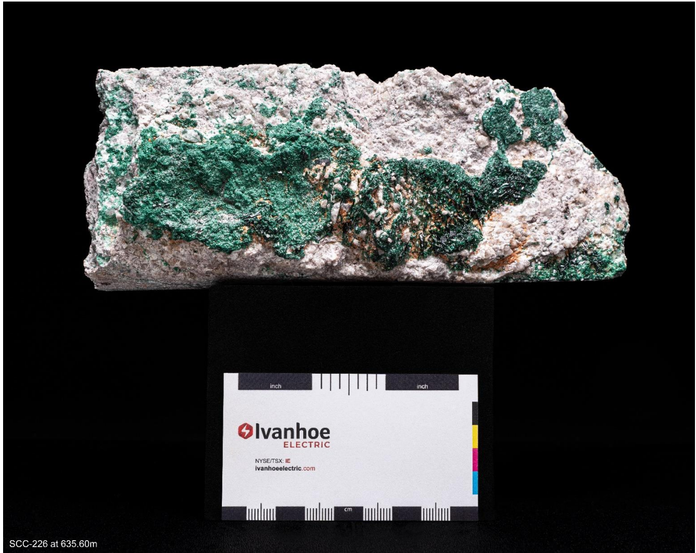
Photo 1: Drill core from Verde Domain drill hole SCC-226 at 635.60 meters showing strong atacamite mineralization (a leachable mineral that is approximately 60% copper by weight) along fractures and within open pockets as blades and rosettes. Assay results for drill hole SCC-226 are pending.
