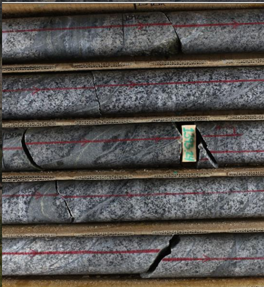
TTD-016: 1391 to 1394m intense sulfide mineralization in vein stockworks
